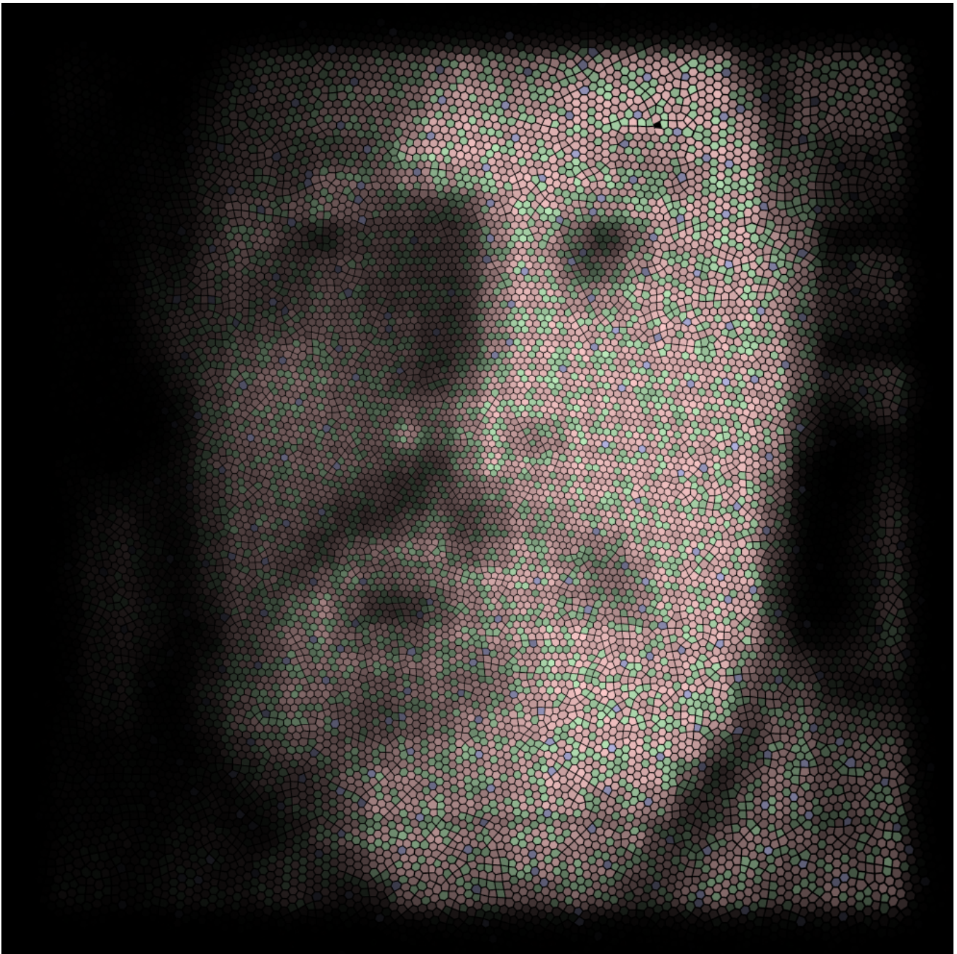
Figure 12: 30×30 pixel display imaged onto synthesized retina. Each 80% fill factor display pixel is visible (broadband light).
